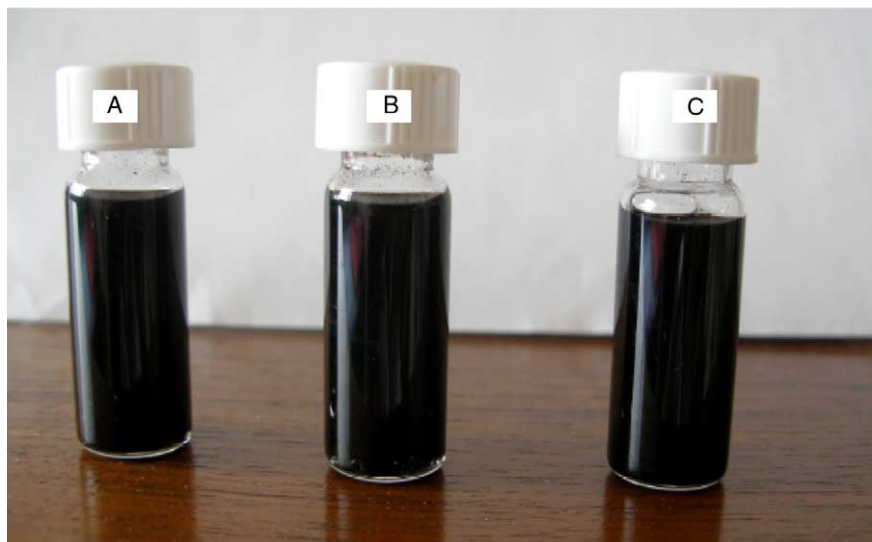
Fig. 10. The glycoconjugates of poly(styrene- alt -maleic acid) wrapped MWNTs in distilled water (A), PBS buffer with pH of 7.4 (B) and DMF (C).
